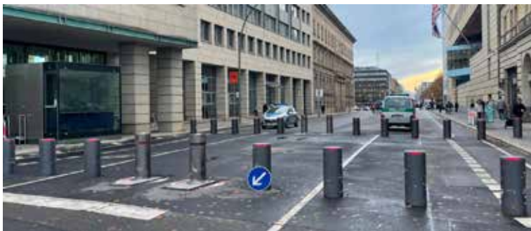
Image 9. An airlock solution in an urban setting – a controlled access point and traffic separation point (Berlin).
