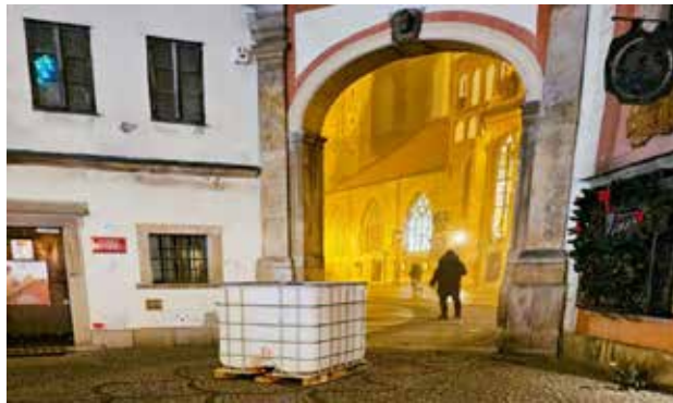
Image 5. An IBC container – element of the traffic management solution that is not a VSB (Poland).
