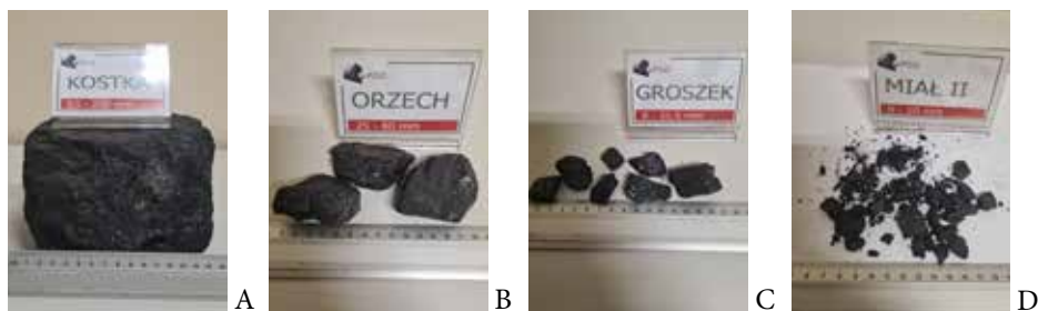
Image 1. Selected hard coal size grades – illustrative photographs: lump coal (A), nut coal (B), pea coal (C), fine coal (D).
