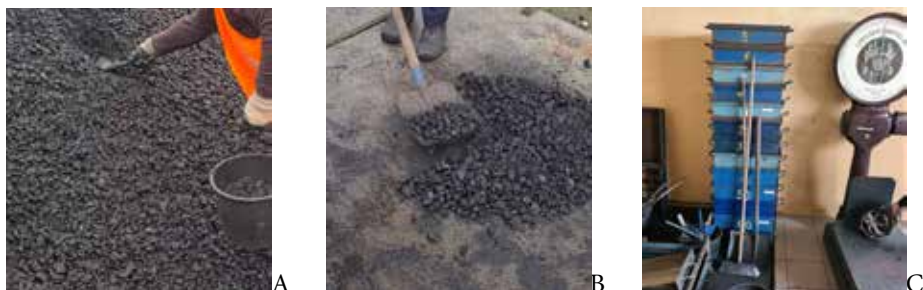
Image 2. Hard coal sampling – illustrative photographs: collection of primary increments (A), quartering (B), nest of sieves for sieve analysis (C).
